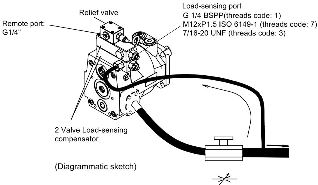
**VA 2-valve load-sensing compensator + Relief valve**
