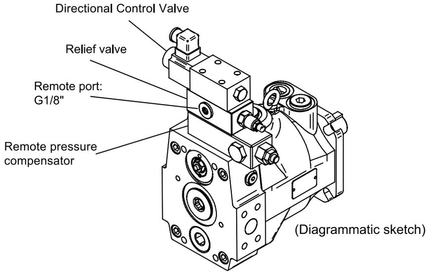
**GR Remote pressure compensator + Electrical unloading**
