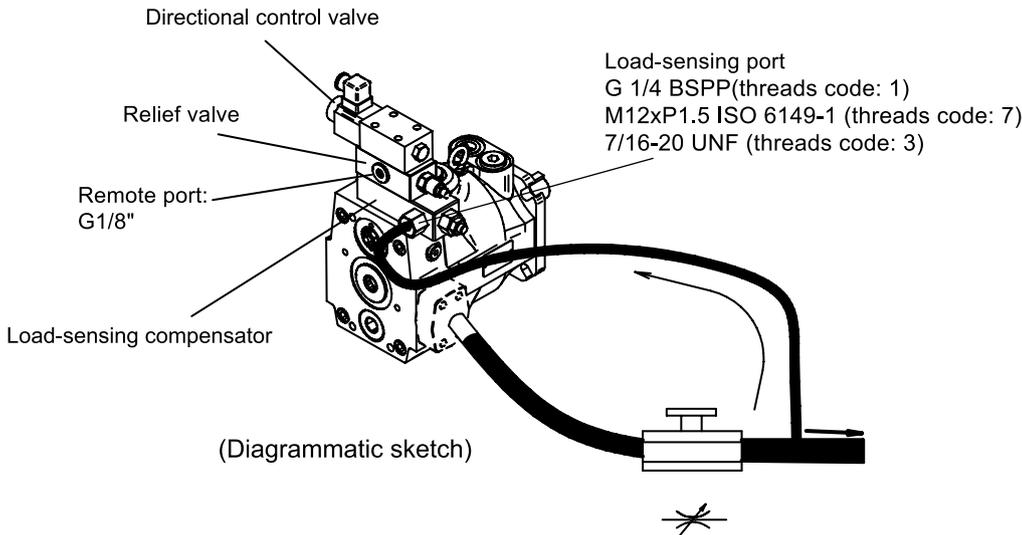
**HR Load-sensing compensator + Electrical unloading**
