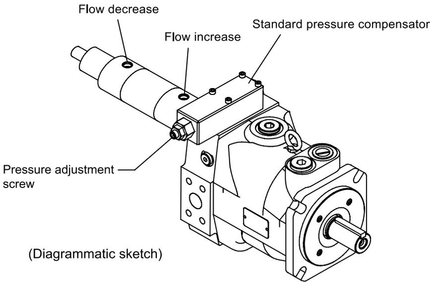
one-stage flow compensator (Cylinder)
