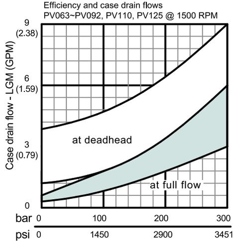
The efficiency and power graphs are measured at an input speed of  $n = 1500$  RPM, a temperature of  $40^{\circ}\text{C}$  and a fluid viscosity of  $46 \text{ mm}^2/\text{s}$ .
