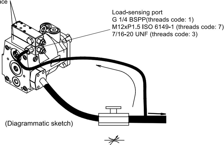
**VM 2-valve load-sensing compensator with NG6 interface**
