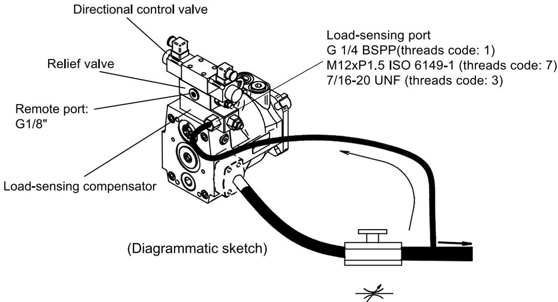
HC Load-sensing compensator
