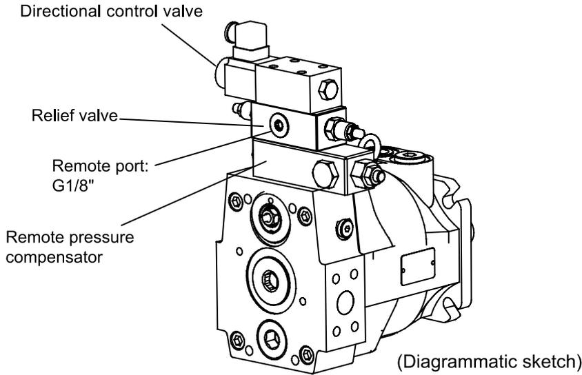
**GB Remote pressure compensator + 2-stage pressure control**
