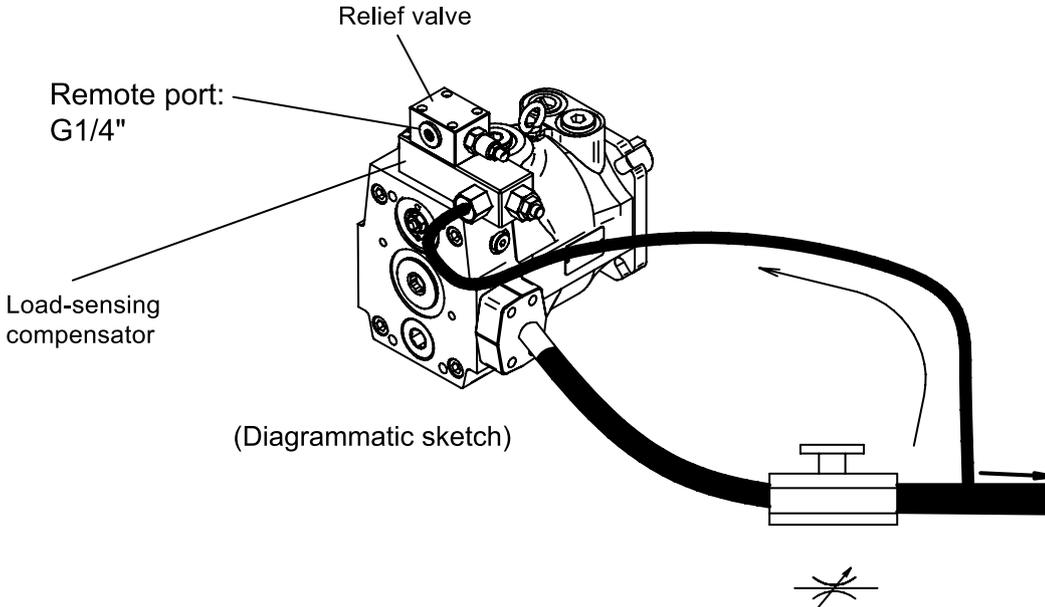
HA Load-sensing compensator + Relief valve
