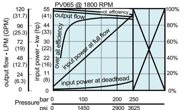
PV032 ~ PV046, PV056, PV065 (Body 2)
