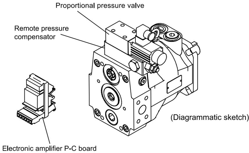
GJ Remote pressure compensator + Proportional pressure valve
