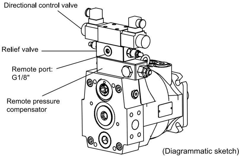
**GC Remote pressure compensator + Electrical unloading + 2-stage pressure control**
