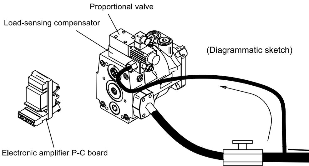
J Load-sensing compensator + Proportional pressure valve
