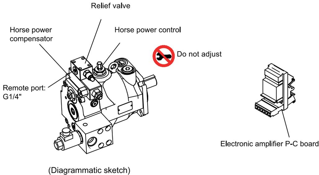
**PQ Horse power load-sensing compensator + Proportional flow valve + Relief valve**
