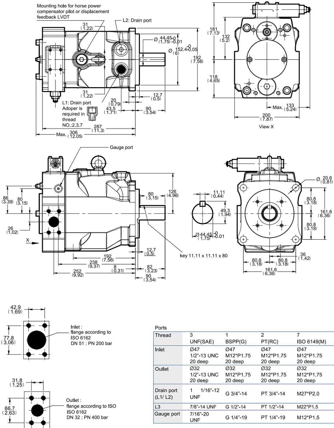
Threads code: 3 & 7 are not standard, not it stock, specially fabricate.
