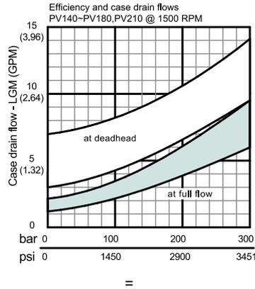
The efficiency and power graphs are measured at an input speed of  $n = 1500$  RPM, a temperature of  $40^{\circ}\text{C}$  and a fluid viscosity of  $46 \text{ mm}^2/\text{s}$ .
