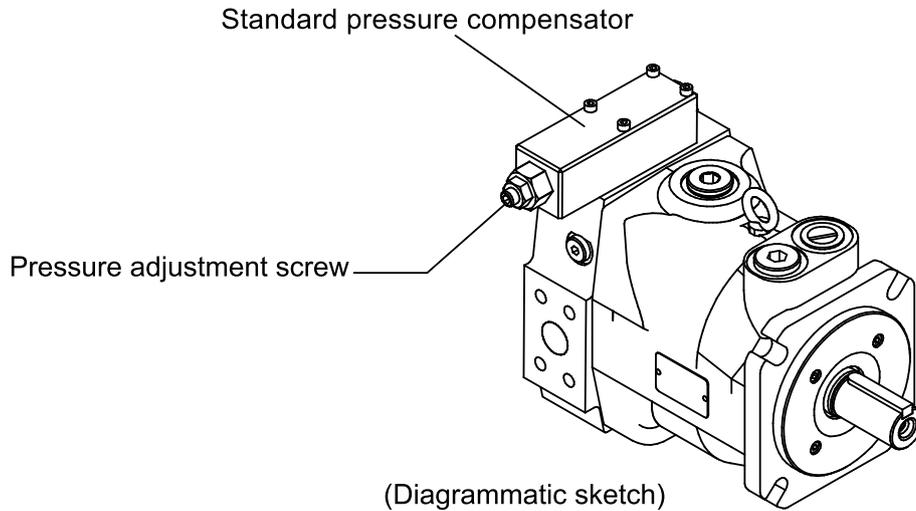
A0 Standard pressure compensator
