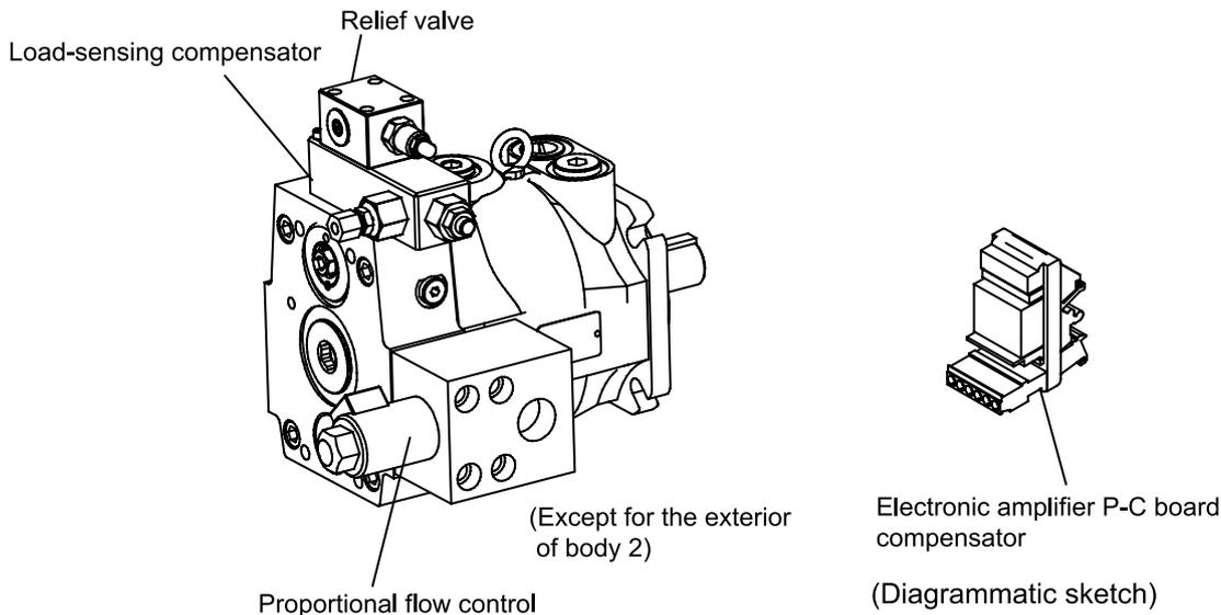
Q Load-sensing compensator + Proportional flow valve + Relief valve
