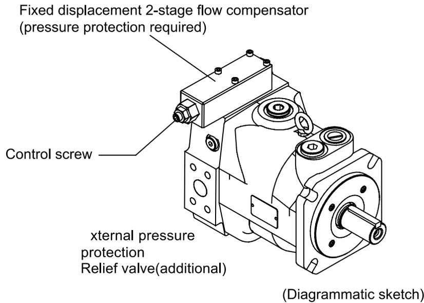
**LC Fixed displacement 2-stage flow compensator**
