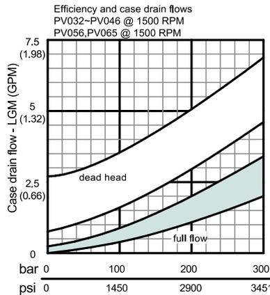
The efficiency and power graphs are measured at an input speed of  $n = 1500$  RPM, a temperature of  $40^{\circ}\text{C}$  and a fluid viscosity of  $46 \text{ mm}^2/\text{s}$ .
